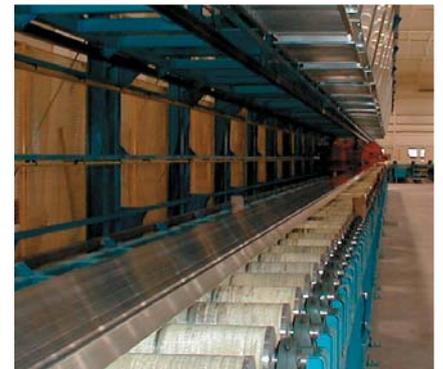
*Runout roller conveyor and overhead air cooling system*
