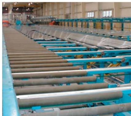
*Saw feed roller conveyor*
