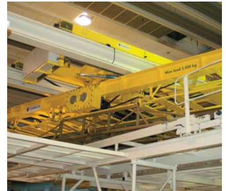
Complete profile baskets handling and packing system
