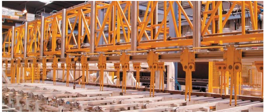
Profile stacker and basket handling system
